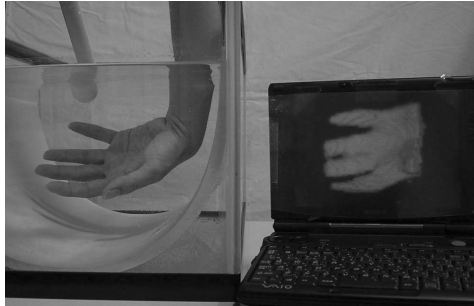
Fig.1. Online IV image: visualizing phantom (human hand) with IV image.
